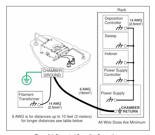
Figure 3-4, Suggested Grounding Connections
