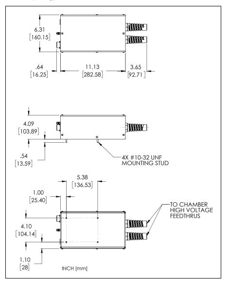
Figure 2-3, ST Filament Transformer Dimensions
