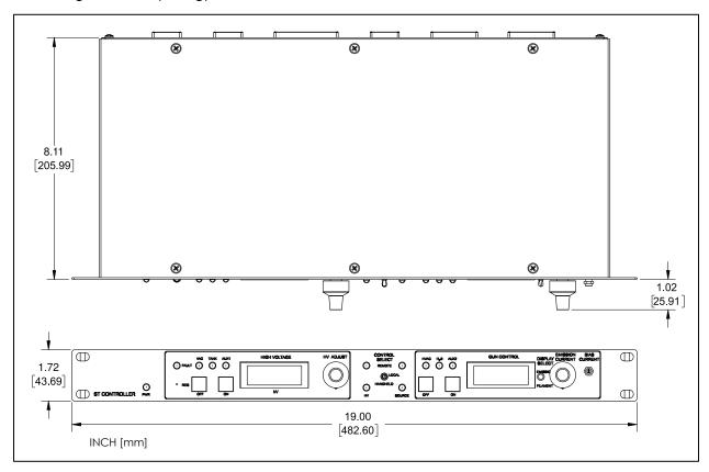
Figure 2-4, ST Controller Dimensions
