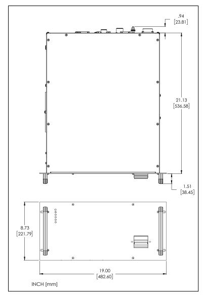
Figure 2-2, ST HVPS Reference Dimensions
