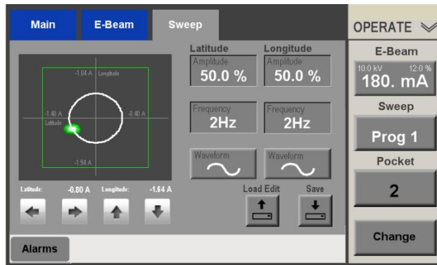
Figure 5-5 Ops>Sweep Screen, Beam and Sweep Both ON
