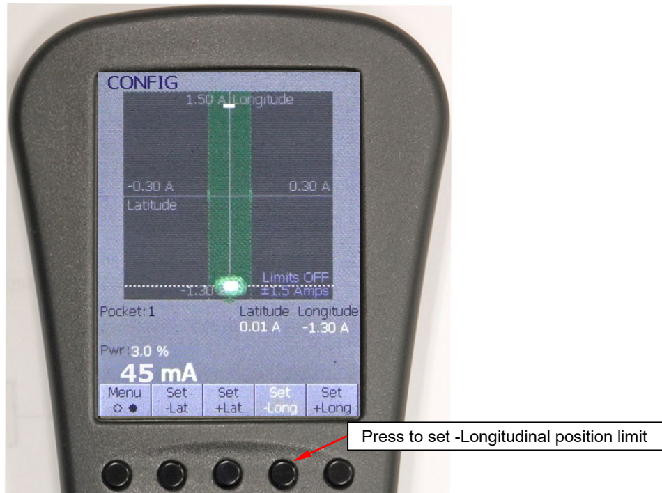
Figure 4-44 Remote Controller Screen After User Sets -Long Beam Position Interlock Limit
