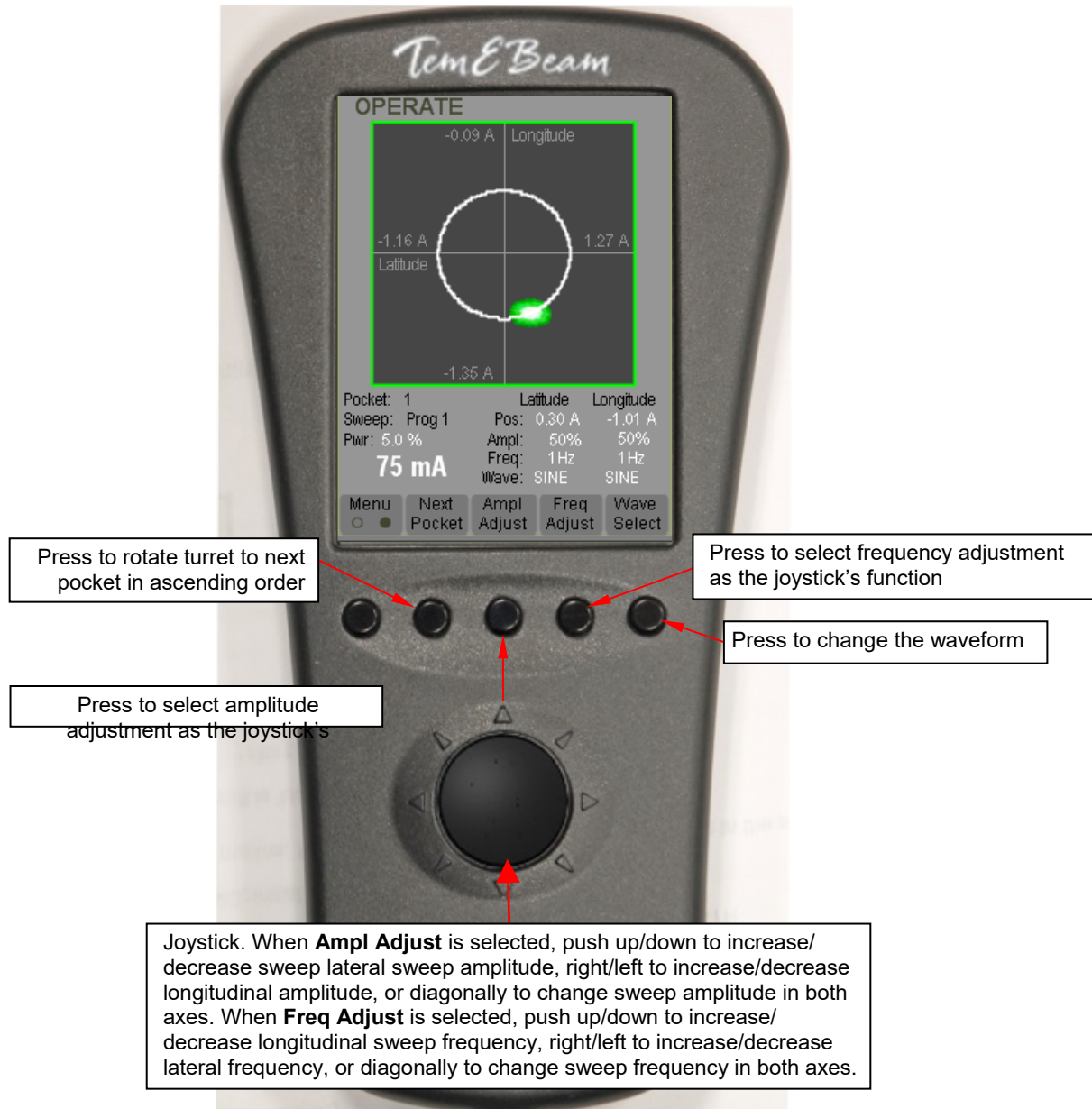
Figure 5-28 Remote Controller’s LOCAL Screen, Menu 2 Selected, Beam and Sweep On
