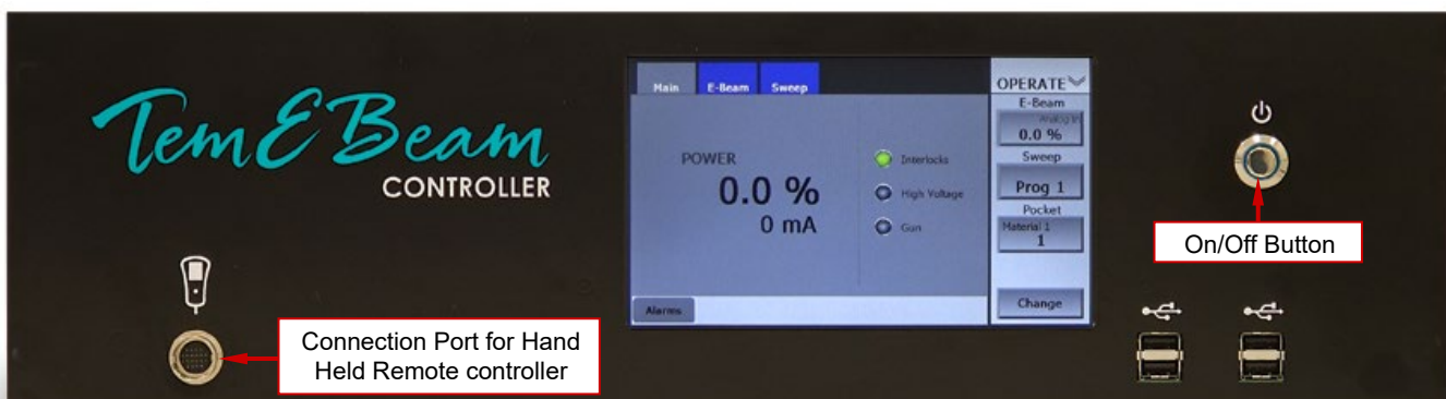
Figure 3-4 EBC Front Panel, Showing Connections Port for Hand Held Remote Controller
