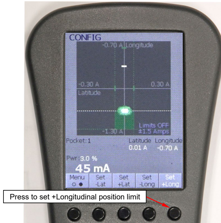
Figure 4-46 Remote Controller Screen After User Sets +Long Beam Position Interlock Limit
