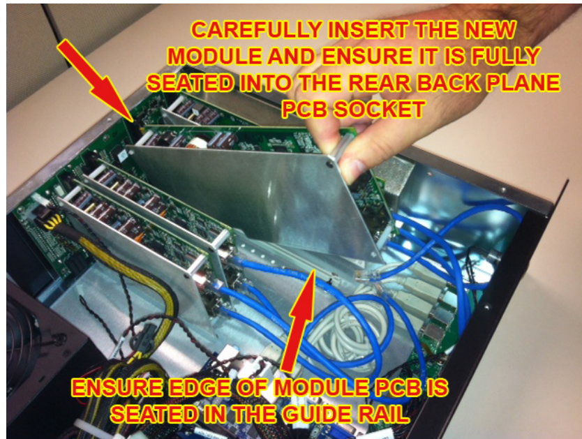
Figure 13-6 Installing the New Control Module
