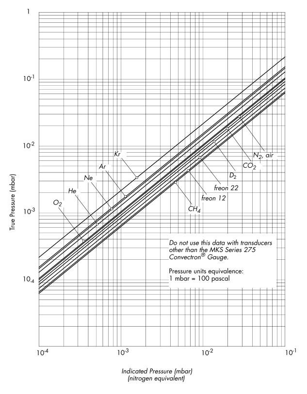
Figure 4-12 Convectron Gauge Indicated vs. True Pressure Curve; 10<sup>-4</sup> to 10<sup>-1</sup> mbar
