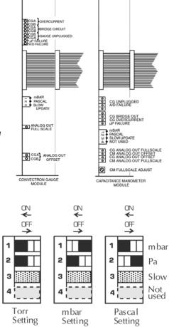
Figure 2-4 Pressure Display Units of Measure Switch Settings
