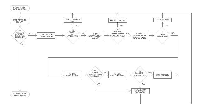
Figure 7-9 Convectron Gauge Display
