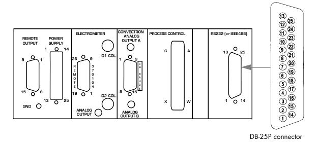
Figure 3-12 Control Unit Rear Panel Showing RS-232 Connector
