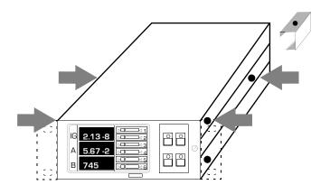
Figure 2-16 Location of Screws for Replacing Top Cover
