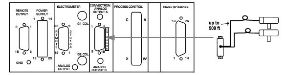
**Figure 3-16** Control Unit Rear Panel Showing the Cable Connection to the Convectron Gauges
