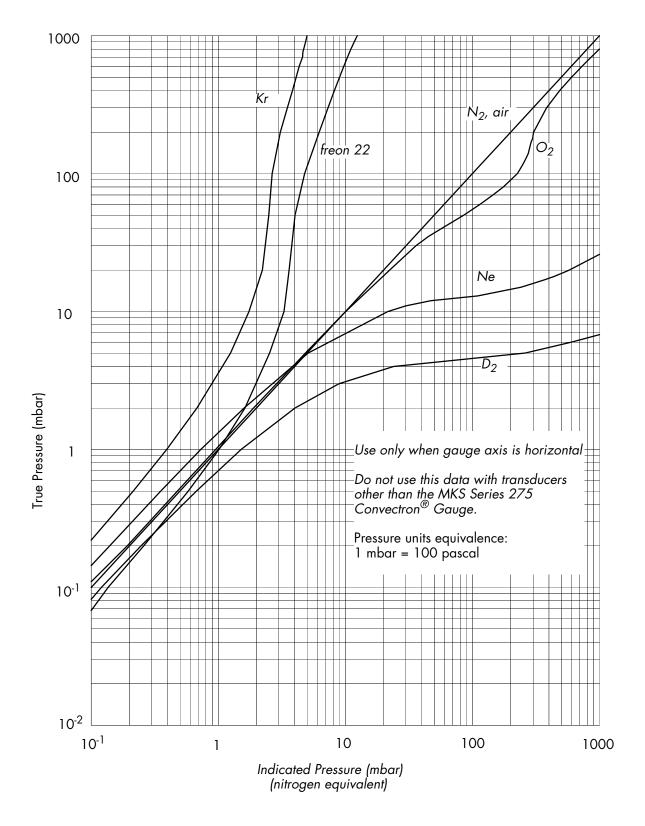
Figure 4-14 Convectron Gauge Indicated vs. True Pressure Curve; 10<sup>-1</sup> to 1000 mbar
