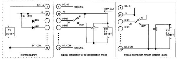
Figure 3-10 Remote Input Connections (Use DA-26P Connector, Supplied)
