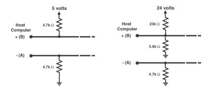
Figure 3-14 RS-485 Bias Resistor
