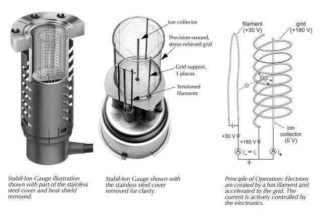
Figure 6-1 Stabil-Ion Gauge Illustrations and Principle of Operation
