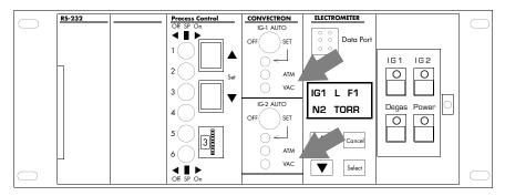
**Figure 4-16** Control Unit Front Panel (with Door Open) Showing Convectron Gauge Zero and Atmospheric Adjustments
