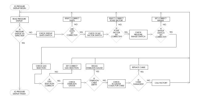
Figure 7-8 Stabil-Ion Gauge Display
