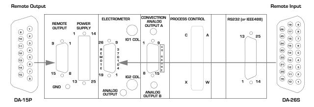
Figure 3-9 Control Unit Rear View Showing Locations of Remote Input and Output Connectors
