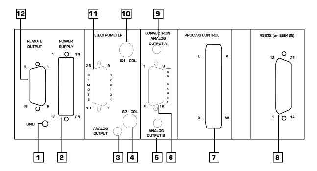
Figure 1-6 Stabil-Ion Vacuum Gauge Control Unit Rear Panel
