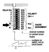
Process Control setpoints 1 (PC1) and 2 (PC2) are controlled by the ionization gauge or gauges. Setpoint 1 operates relay 1. Setpoint 2 operates relay 2. Relays 1 and 2 are also shown as K1 and K2 on the printed circuit board for reference during IG assignment. IG1, IG2, or both can be assigned to operate either setpoint 1 or 2. Use Table 2-2 to assign the IG's to the setpoints.
