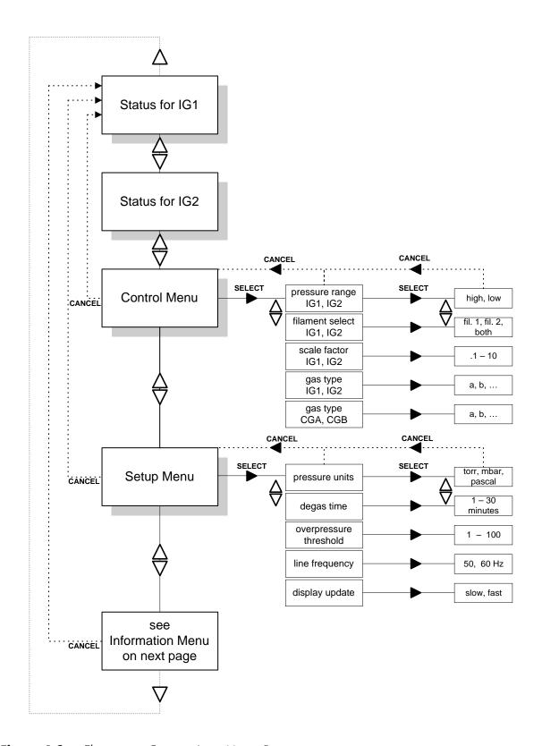
Figure 4-3a Electrometer Function Input Menus Diagram
