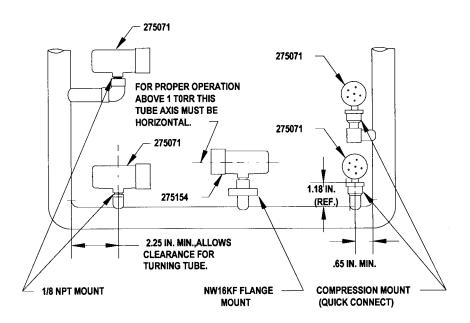
Figure 3-3 Convectron Gauge Installation
