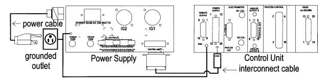
Figure 3-19 Power Supply and Control Unit Rear Views Showing Power Cable Connections
