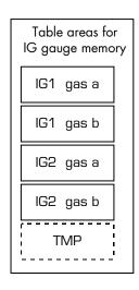
The numbers in the display correspond to the Serial Tag Numbers on the Stabil-Ion Gauge tubes. The way to change data from TMP to IG2 gas table location is as follows:
