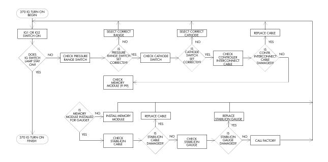
Figure 7-7 Stabil-Ion Gauge Turn ON
