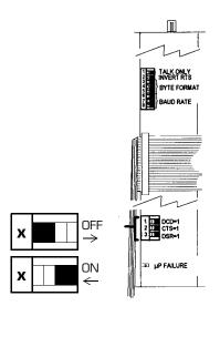
Figure 2-13 Top View of RS-232 Module
