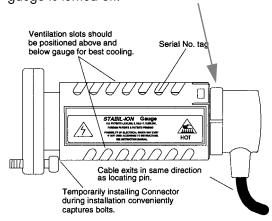
**Figure 3-2** Stabil-lon Gauge with Connector and Guard
