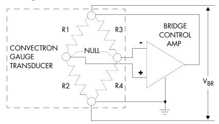
Figure 6-2 Simplified Schematic of Convectron Gauge
