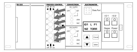
Front Panel of Control Unit (with Door Open) Figure 3-8 Showing Locations of Override Switches
