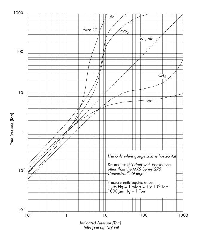
Figure 4-10 Convectron Gauge Indicated vs. True Pressure Curve; 10<sup>-1</sup> to 1000 Torr
