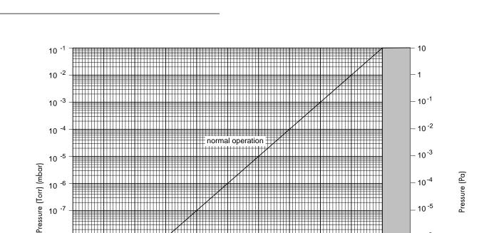
Figure 4-8 Ionization Gauge Analog Output vs. Pressure
