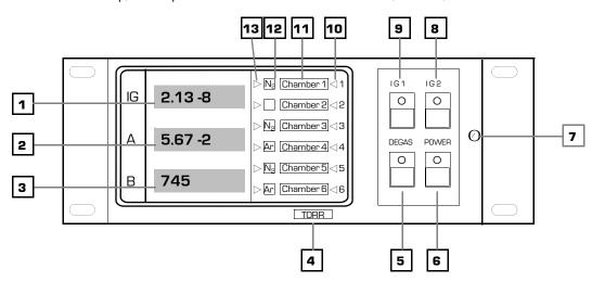
Figure 1-4 Stabil-Ion Vacuum Gauge Control Unit Front Panel
