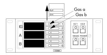
**Figure 4-5** Control Unit Front Panel Showing Removal of Units of Measure Label Card
