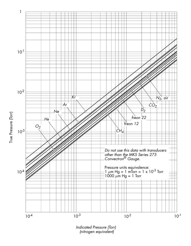
Figure 4-9 Convectron Gauge Indicated vs. True Pressure Curve; 10<sup>-4</sup> to 10<sup>-1</sup> Torr
