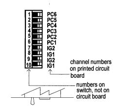
Partial Top View of Process Figure 2-9 Control Module
