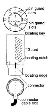
**Figure 3-18** Stabil-lon Gauge connector orientation (prior to installation)
