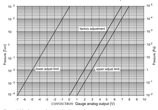
Figure 4-18 Convectron Gauge Analog Output vs. Pressure
