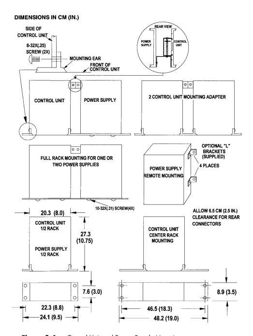
Figure 3-4 Control Unit and Power Supply Mounting
