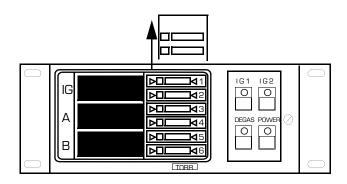
**Figure 2-5** Control Unit Front Panel Showing Removal of Units of Measure Label Card
