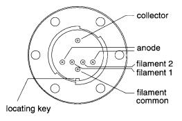
Figure 3-1 Stabil-Ion Gauge Pin and Locating Key Locations
