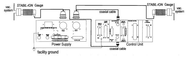
**Figure 3-17** Power Supply and Control Unit Rear Views Showing the Cable Connections to the Stabil-Ion Gauges
