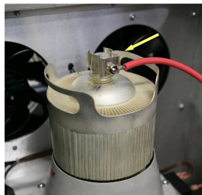
Figure 4-G Anode Connection clipped to power tube, left TT-10/15/20, right TT-8
