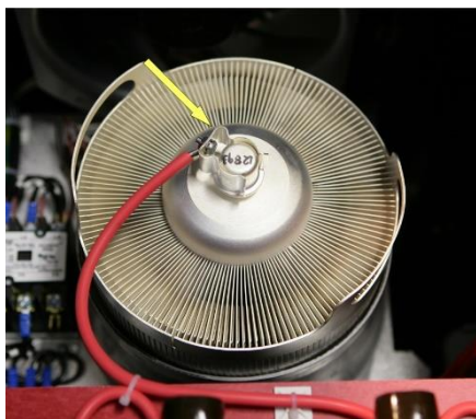
Figure 4-G Anode Connection clipped to power tube, left TT-10/15/20, right TT-8
