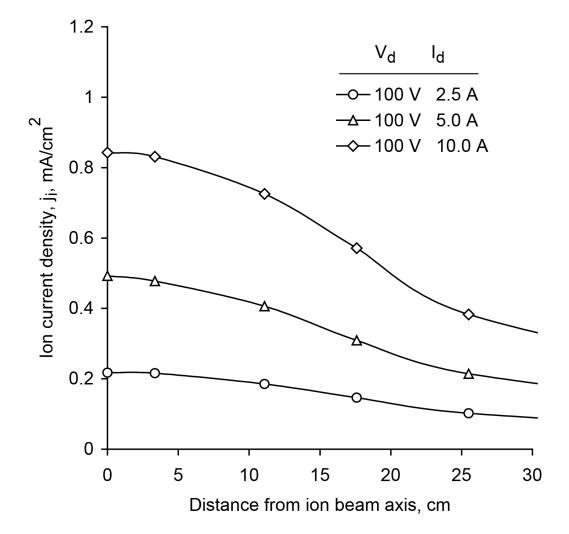
Figure 6-24. Flat target ion current density profiles for the KRI<sup>®</sup> eH2000HC ion source. Source to target distance is 30 cm (12 in.) and normal to beam axis. The working gas is nitrogen.
