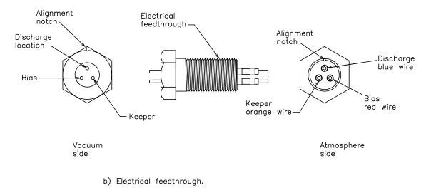
Figure 2-6. 1 inch bolt feedthrough details.
