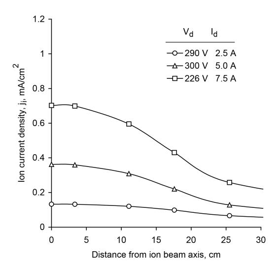
Figure 6-28. Flat target ion current density profiles for the KRI<sup>®</sup> eH2000HC ion source. Source to target distance is 30 cm (12 in.) and normal to beam axis. The working gas is nitrogen.
