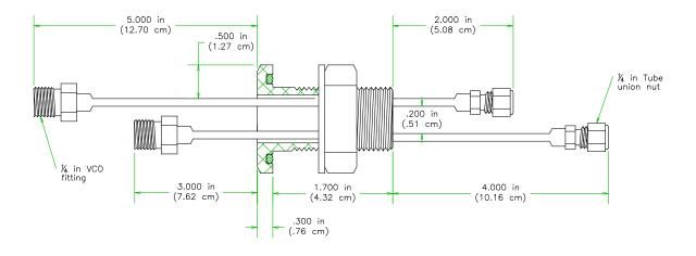
b) 1 inch bolt water feedthrough
