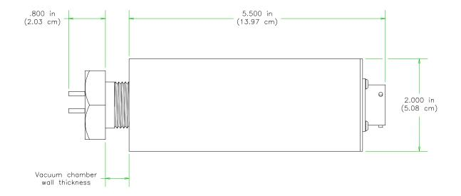
Figure 2-5. 1 inch bolt feedthrough dimensions.
