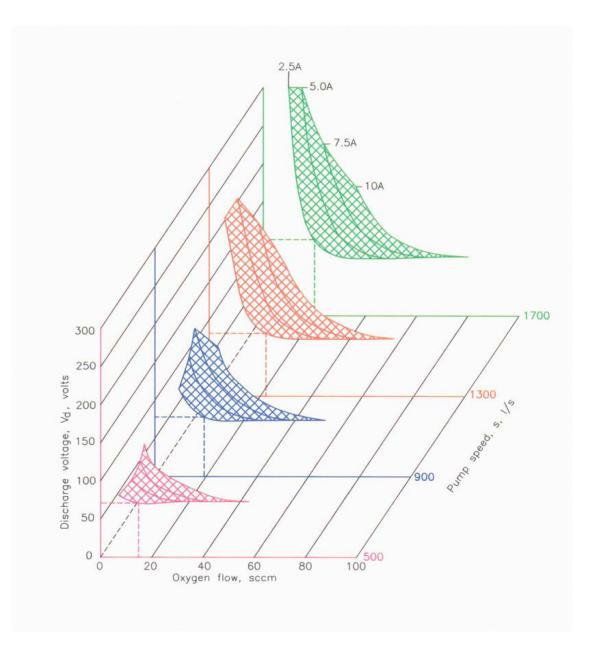
Figure 6-3. Range of operation for the KRI<sup>®</sup> eH2000HC ion source at various pump speeds, using oxygen.
