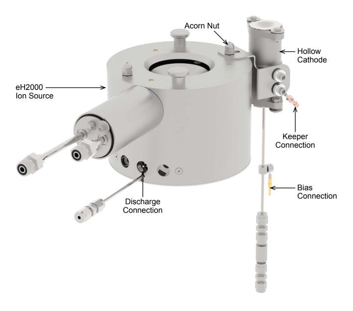
Figure 2-16. Hollow cathode mounting and connections
