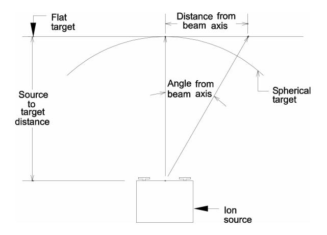
Figure 6-10. Spherical and flat target configurations.
