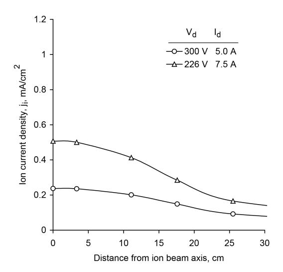
Figure 6-16. Flat target ion current density profiles for the KRI<sup>®</sup> eH2000HC ion source. Source to target distance is 30 cm (12 in.) and normal to beam axis. The working gas is argon.
