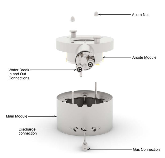
Figure 2-1. The eH2000HC water-cooled anode ion source with the anode module removed.
