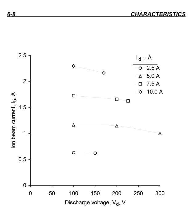
Figure 6-5. Variation of ion beam current with discharge voltage at various discharge currents, using argon.
