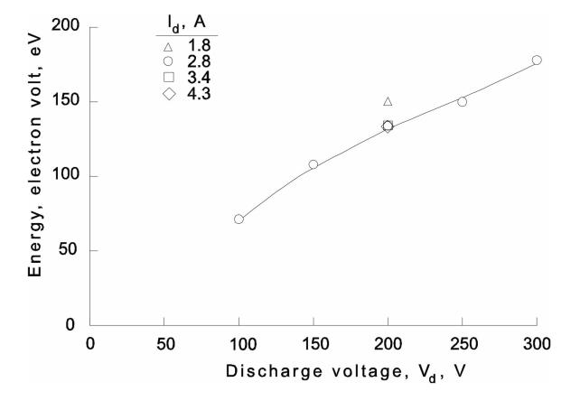
Figure 6-8. Mean ion energy with variation in discharge voltage.
