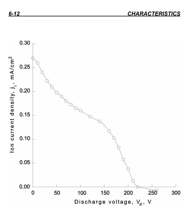
Figure 6-9. Retarding potential probe analysis of the ion beam at a discharge voltage and current of 200 V and 2.8 A.
