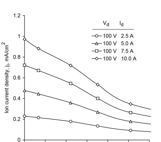
Figure 6-18. Flat target ion current density profiles for the KRI<sup>®</sup> eH2000HC ion source. Source to target distance is 30 cm (12 in.) and normal to beam axis. The working gas is oxygen.
