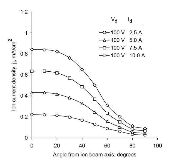
Figure 6-11. Spherical ion current density profiles for the KRI<sup>®</sup> eH2000HC ion source with the source at the center of the sphere. Source to target distance is 30 cm (12 in.). The working gas is argon.
