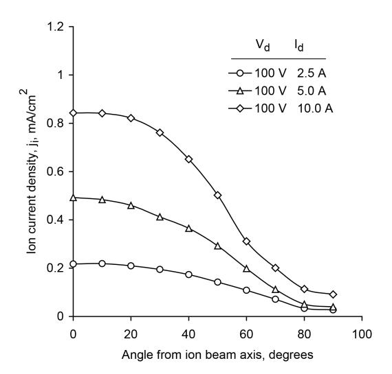
Figure 6-23. Spherical ion current density profiles for the KRI<sup>®</sup> eH2000HC ion source with the source at the center of the sphere. Source to target distance is 30 cm (12 in.). The working gas is nitrogen.
