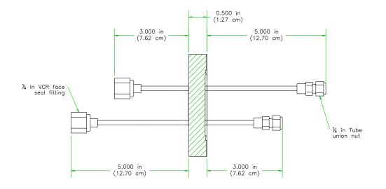
a)  $2\frac{3}{4}$  inch CF flange gas feedthrough
