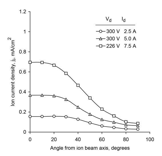
Figure 6-21. Spherical ion current density profiles for the KRI<sup>®</sup> eH2000HC ion source with the source at the center of the sphere. Source to target distance is 30 cm (12 in.). The working gas is oxygen.
