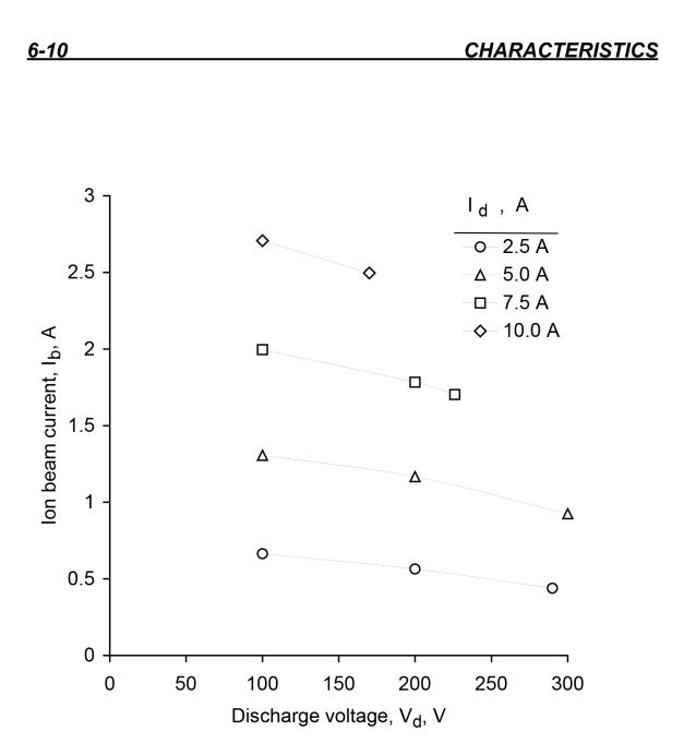
Figure 6-7. Variation of ion beam current with discharge voltage at various discharge currents, using nitrogen.
