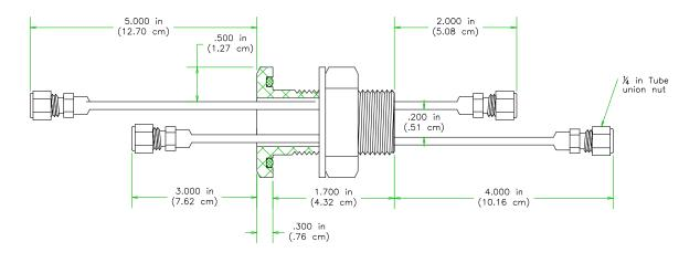
b) 1 inch bolt gas feedthrough
