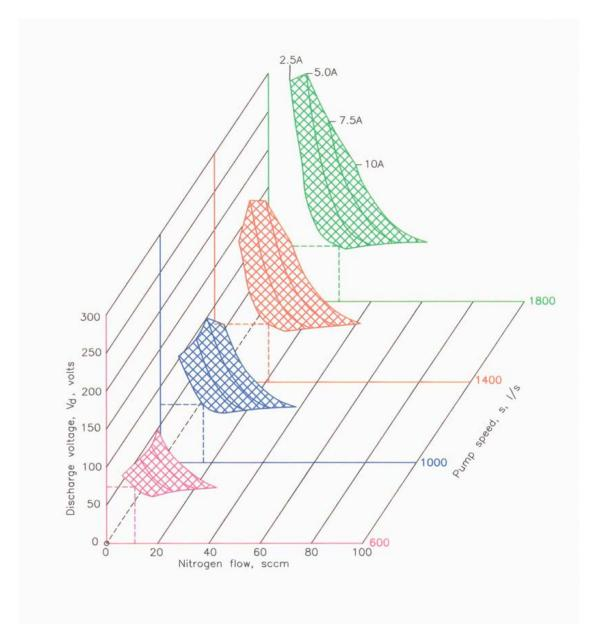
Figure 6-4. Range of operation for the KRI<sup>®</sup> eH2000HC ion source at various pump speeds, using nitrogen.
