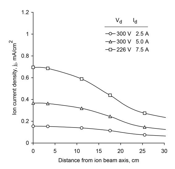
Figure 6-22. Flat target ion current density profiles for the KRI<sup>®</sup> eH2000HC ion source. Source to target distance is 30 cm (12 in.) and normal to beam axis. The working gas is oxygen.
