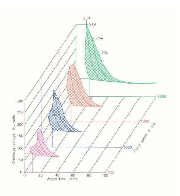
Figure 6-2. Range of operation for the KRI<sup>®</sup> eH2000HC ion source at various pump speeds, using argon.
