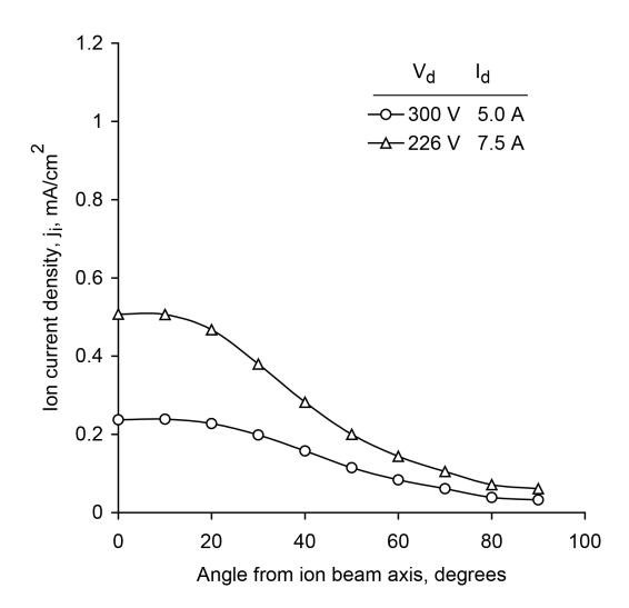
Figure 6-15. Spherical ion current density profiles for the KRI<sup>®</sup> eH2000HC ion source with the source at the center of the sphere. Source to target distance is 30 cm (12 in.). The working gas is argon.
