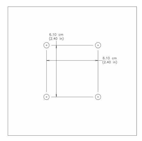
Figure 2-15. Mounting hole locations for the (optional) transit support.
