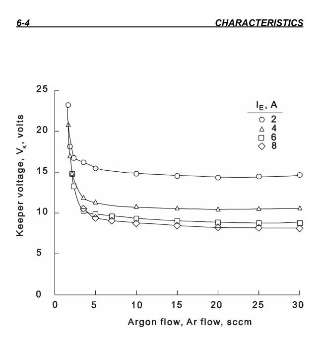
Figure 6-1. Variation in hollow cathode keeper voltage with argon gas flow for various emission currents.
