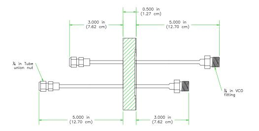
a)  $2\frac{3}{4}$  inch CF flange water feedthrough
