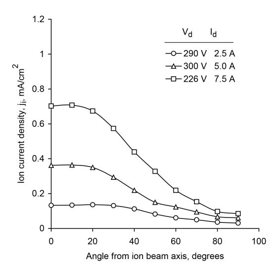
Figure 6-27. Spherical ion current density profiles for the KRI<sup>®</sup> eH2000HC ion source with the source at the center of the sphere. Source to target distance is 30 cm (12 in.). The working gas is nitrogen.
