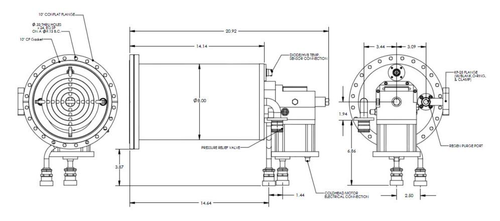
Figure 1 – Cryo-Plex 8 Cryopump with CF Inlet Dimensions
