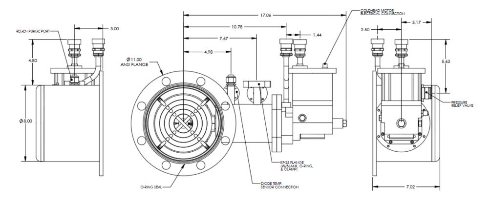
Figure 2 – Cryo-Plex 8LP Cryopump with ANSI Flange Dimension
