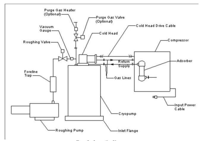
Figure 3 – Connection Diagram
