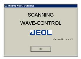
OK Clicking on this button opens the SCANNING window (Normal mode setting).
